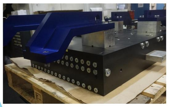
The cooling block feet are also coated. They are milled from solid aluminium and allow for an abrasion-resistant, coloured coating that is sustainable for years.
