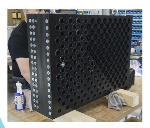
The cooling block in particular is treated INSIDE in all bores and channels. This means that the cooling water is not contaminated with oxidised aluminium, the cooling efficiency is maintained and cooling sleeves can be easily removed after years.
