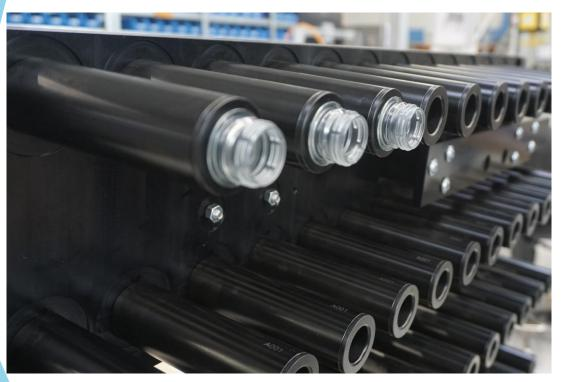
All other parts of the cooling stations are also coated for the reasons mentioned. This coating is hard and abrasion-resistant, which provides very good protection, especially against corrosion.
