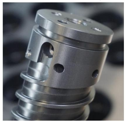
A cooling channel which is serial drilled with the spiral channel in the bottom area ensures intensive cooling at the critical preform bottom (gate area) in order to minimise the formation of crystallinity in the cooling phase and to produce optimum preforms for the blowing process
