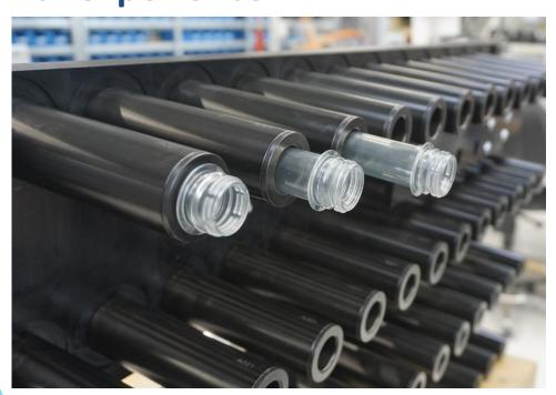
ReduPET GmbH has more than 20 years of experience in cooling sleeve design for singlestage and two-stage production systems, an optimal basis for efficient cooling of preforms to achieve optimal cycle times.
