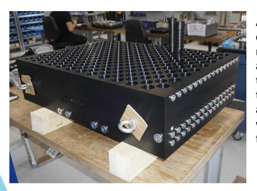
All aluminium parts of the entire cooling station are made corrosion-resistant and abrasion-proof by a special treatment. This means that the unit does not corrode and remains clean for years, which is necessary in the food industry.
